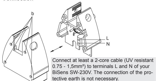
1. Remove the wall fixing screws (b) of the BiSens SW-230V.
